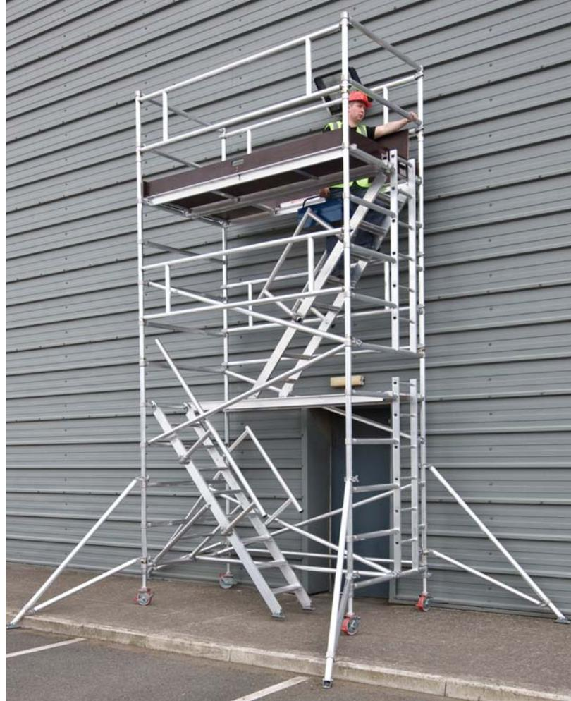
**The Instant Stairway tower is a versatile unit which can easily convert both a standard Span 300 and a Span 400 mobile access tower into a stairway tower. It provides safe landings every 2 metres. Stairway steps are 145mm deep, with a clear width of 450mm making it easy to carry tools. The step rise is 230mm and the angle of inclination is 51 degrees.**
